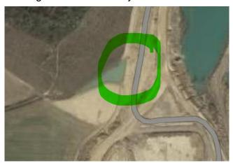
Water is currently ponding west of the access road, once again it appears the drain under the road is not low enough to prevent ponding of water. This area should drai to New Field Lagoon.
